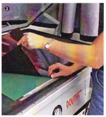
Place the flat on top of the plate in the vacuum frame.
