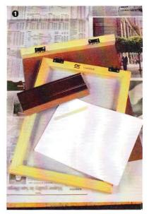
A printing board is a piece of wood about 3 inches wider all around than your screen. Attach it with hinges to one end of your frame. For a smoother printing surface, tape poster board or untextured mat board over the wood.
