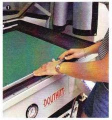
Insert the plate into the vacuum frame.
