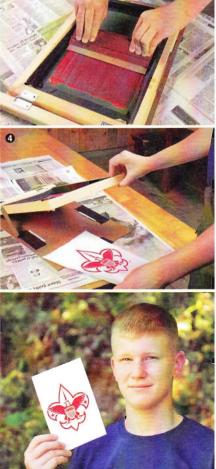
**Step 3**—After completing the print stroke, lift the screen frame off the surface and return the squeegee to the top of the frame, using a flood stroke to spread a thin film of ink and prevent the screen from drying out and blocking fresh ink. (Some screens have a leg to hold the frame up between prints, or you can prop it with a small block of wood.)
